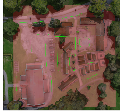
Fig. 4: Top-down view of the Village area. The red bounding box illustrates the volume to be explored. The area is roughly 1 hectare and populated with multiple dynamic obstacles. The paths of the dynamic obstacles are highlighted in green where the lines indicate that the dynamic obstacle moves back and forth while a loop indicates that the dynamic obstacles circulate.
